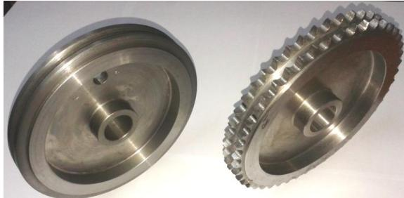
Fig. 12: The blank and the sprocket-completed
