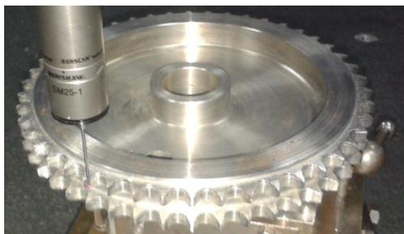
Fig. 13: Image from during performs of automated scanning of the sprocket profile
