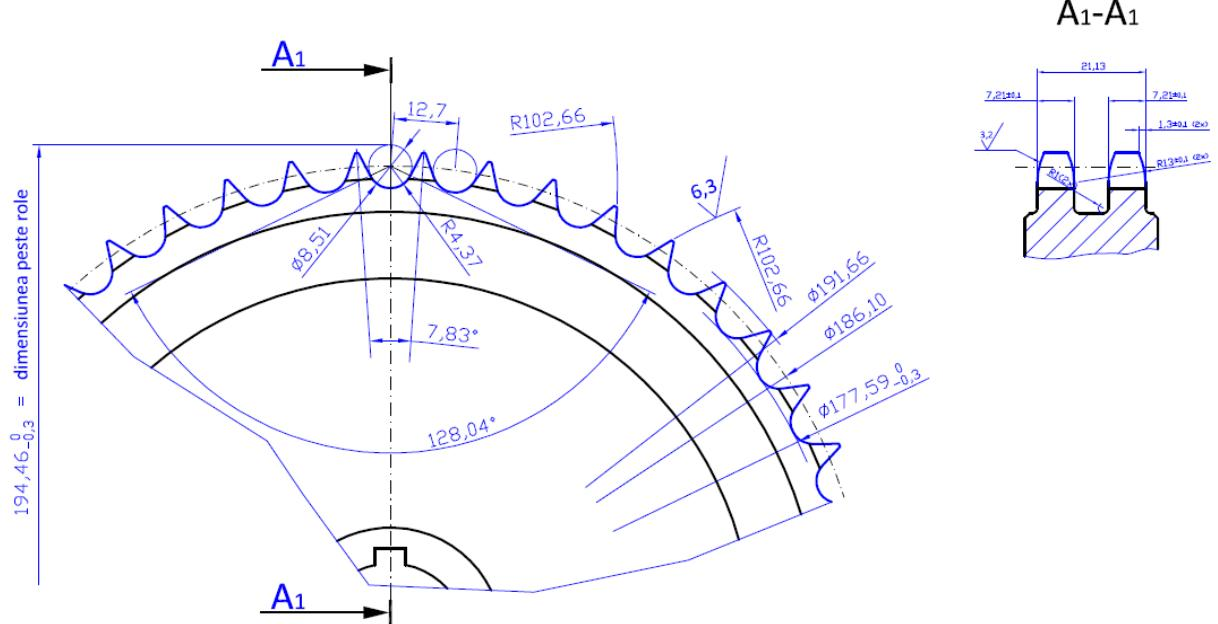
Fig. 2: Double profile of studied sprocket
