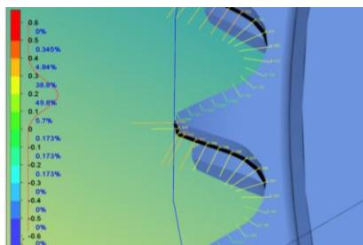
Fig. 18: The color graph of the scanning „SCN<sub>2</sub>” of the profile 1 of sprocket with double tooting
