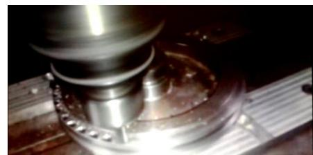
Fig. 7: Milling of first addition of processing at the double sprocket profile
