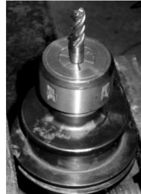
Fig. 3: End mill characteristics used at machining of the profile are  $\phi = 8$  [mm] and  $z = 4$  [teeth]
