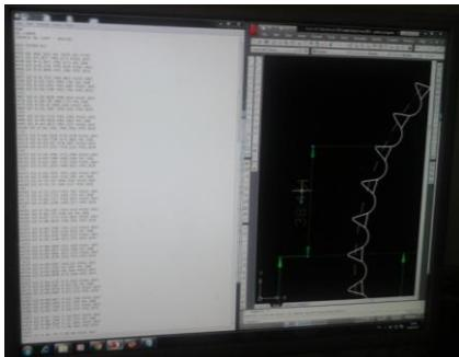
Fig. 4: Introduction of G codes in processing program, simultaneously with determining points on tooth profile
