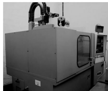
Fig. 1: „AXA VSC 0-500M” Controlled Vertical Machining Center [2]
