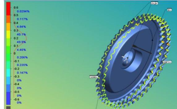
Fig. 20: - The graph of the profile deviation on the double toothed of the sprocket, in overall
