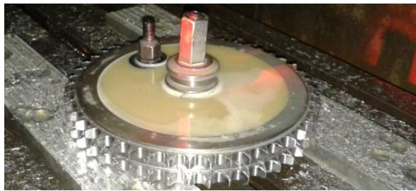
Fig. 11: Double toothed of sprocket in final stage of execution
