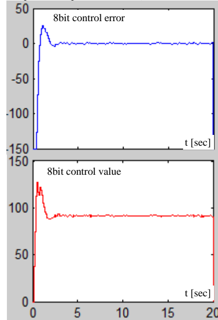
Fig. 8: Error and control signal (forward discretization).
