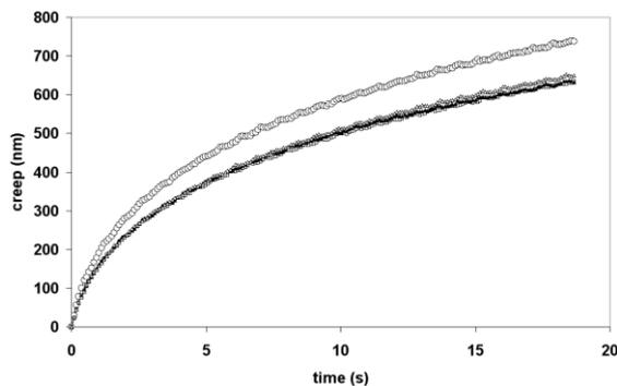
Fig. 7. Indentation creep response for UHMWPE (circles) and PIII-UHMWPE (other symbols)
