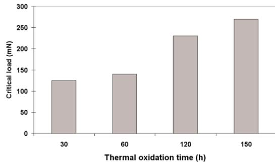
Fig. 11. Variation in critical load with thermal treatment time for thermal oxidation of FeAl.
