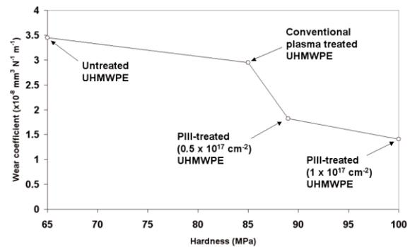
Fig. 8. Correlation between the wear rate (pin-on-disk tribometer) and hardness for UHMWPE after various plasma treatments
