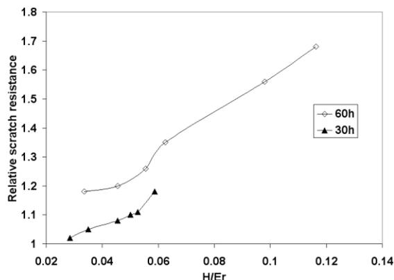
Fig. 12. Variation in the relative wear resistance with  $H/E_r$  for 30 and 60h thermal oxidation treatment FeAl.
