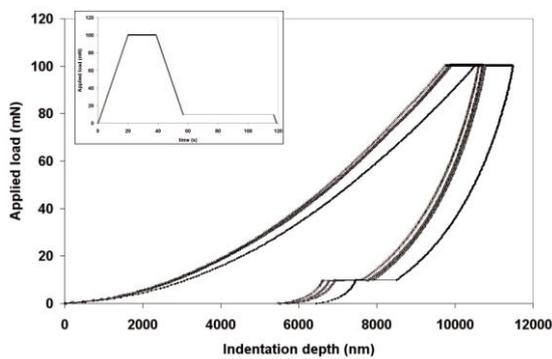
Fig. 10. Nanoindentation to 100 mN on UHMWPE (filled) and PIII-UHMWPE (other symbols). The insert shows the load history with hold periods at 100% of peak load (for creep assessment) and at 90% unloading (to assess creep recovery)
