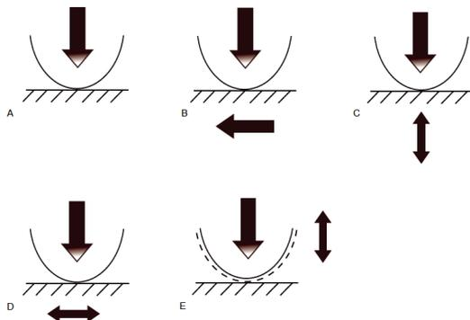
Fig. 2. Contact geometries in nanomechanical testing (a) indentation (b) scratch/wear (c) impact/contact fatigue (d) fretting and reciprocating wear (e) impulse impact
