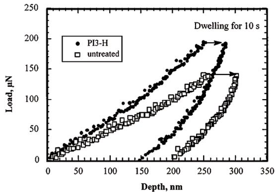
Fig. 6. Nanoindentation of UHMWPE and PIII-UHMWPE. Reprinted with permission from *J. Mater. Sci. Lett.* 19 (2000) 1147
