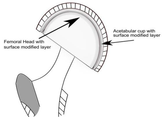
Fig. 4. Surface engineered hip joint prosthesis
