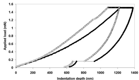
Fig. 9. Nanoindentation of UHMWPE (triangles) and He-modified UHMWPE (circles)
