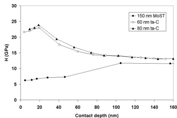
Fig.1. Variation in hardness with contact depth for 150 nm MoST, 60 nm ta-C and 80 nm ta-C on Si
