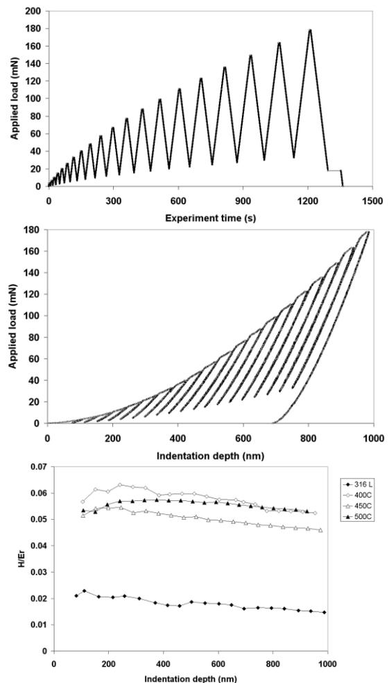
Fig. 5. (a) load vs. time for load partial unload experiment on plasma carburized steel; (b) Typical load-partial unload nanoindentation behaviour on sample plasma carburized at 500 °C for 15 hr; (c) Variation in the ratio H/E<sub>r</sub> with contact depth for untreated 316 stainless steel and samples after carburization.
