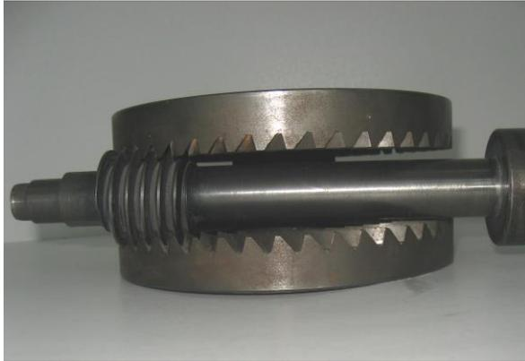
**Fig. 4.** Dual worm face gear with cylindrical pinion
