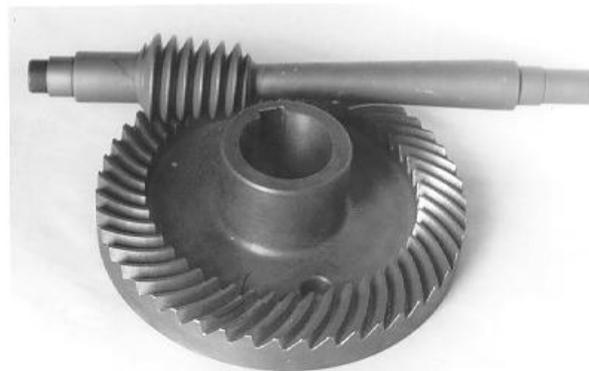
**Fig. 2.** Worm face gear with tapered pinion
