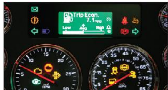
Figure 5. Cummins Road Relay display
