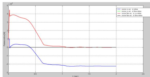
**Fig. 4.** Evolution of active power transit between the hybrid system based on renewable energy sources and the public network
