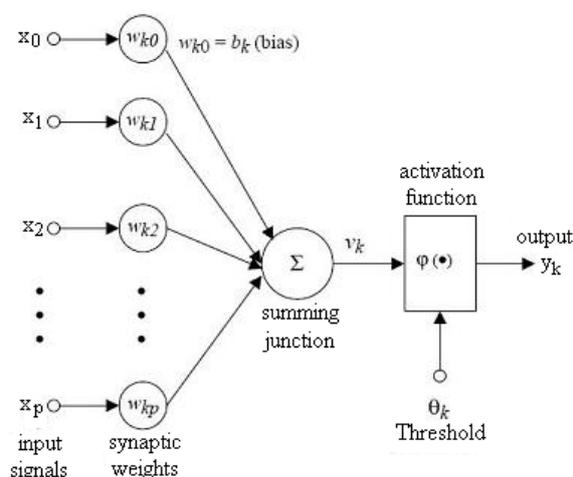
Fig. 2. Structure of an artificial neural network.
