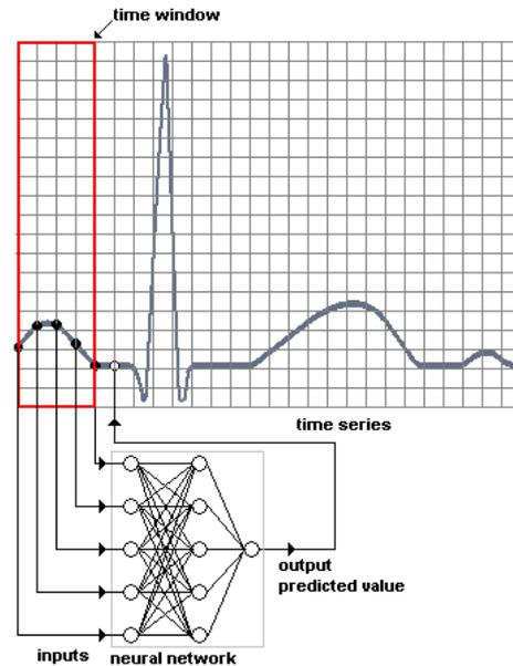
Figure 5. The principle of estimation
