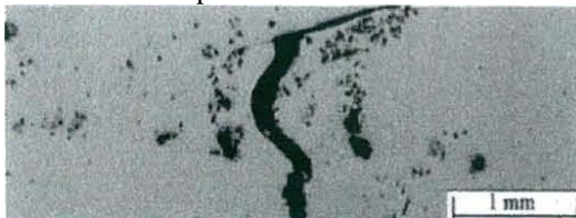
Fig. 4. Leaker in the section of an aluminium diecast part
