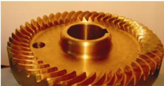
Fig. 3 The worm-wheel with reverse tapered
