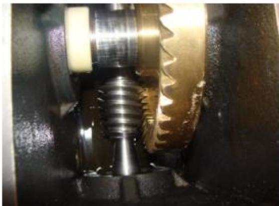
*Fig. 1 Worm face-gear with reverse tapered pinion*
