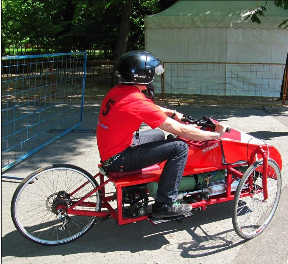
*Fig. 8 The experimental pneumatic vehicle*
