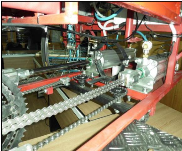
*Fig. 4 The engine of the vehicle*
