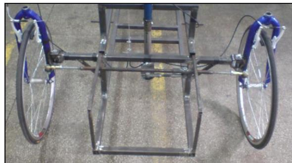
Fig. 2 The steering mechanism
