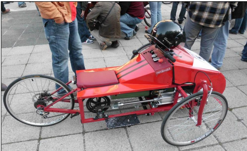
Fig. 7 The pneumatic vehicle
