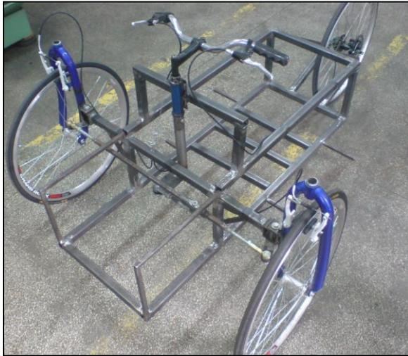
*Fig. 3 The assembled chassis*
