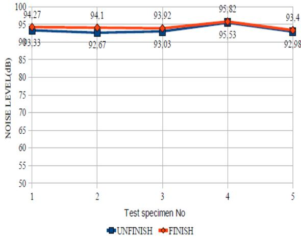
**Figure 5: Noise level chart of 10 degree flanks**
