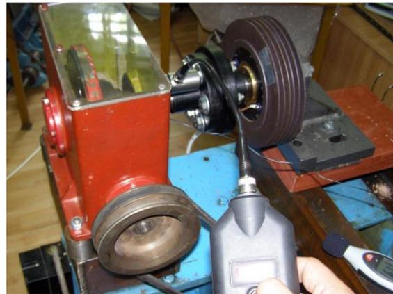
**Figure 4 – Test gear box with test instrumentation**
