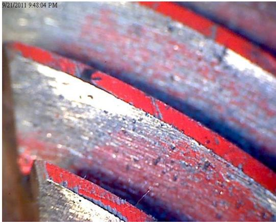
**Figure 9 : Scratches was effective removed**
