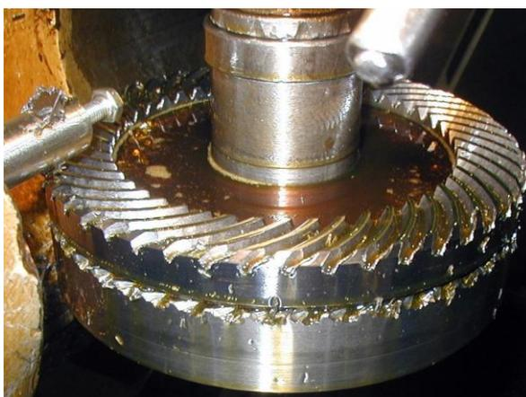
**Figure 1: Hobbing of worm plain wheels by fly cutters**
