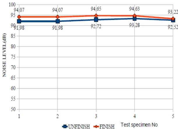
**Figure 6: Noise level chart of 30 degree flanks**
