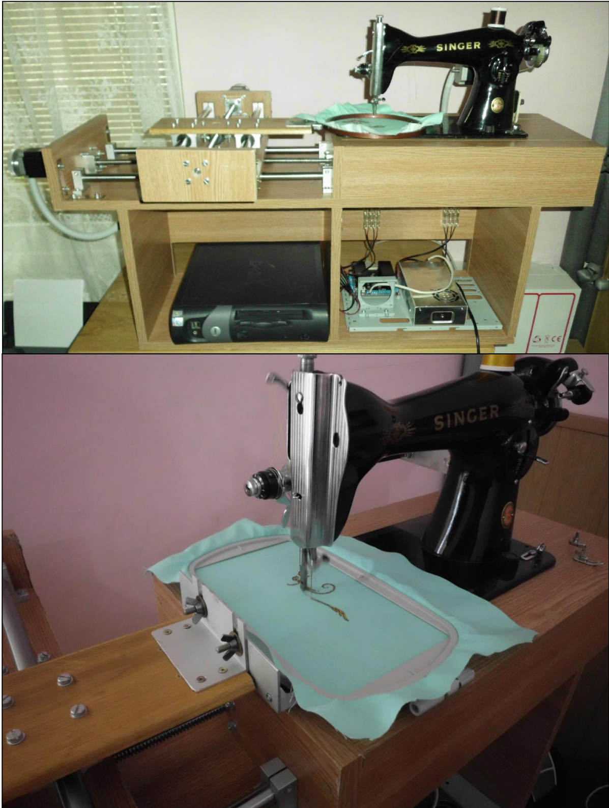
Fig. 8. The CNC sewing and embroidery Machine
