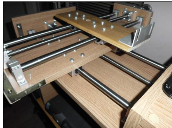
Fig. 3. The linear translation stages
