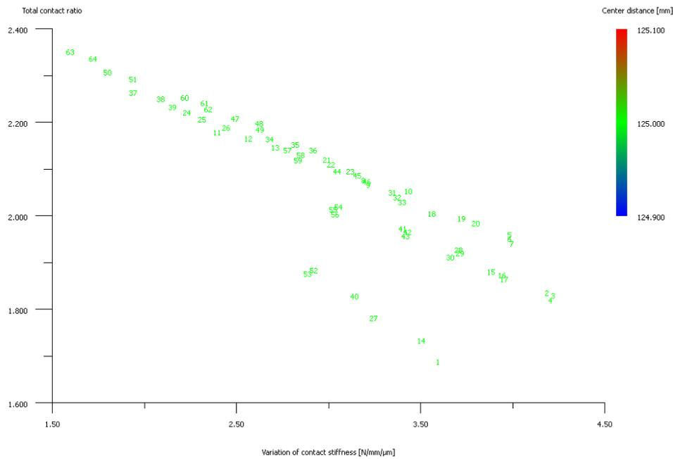
**Fig.11. Variation of contact stiffness / total contact ratio**
