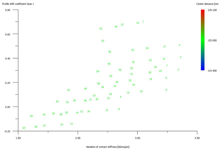
**Fig.10. Variation of contact stiffness / profile shift coefficient**
