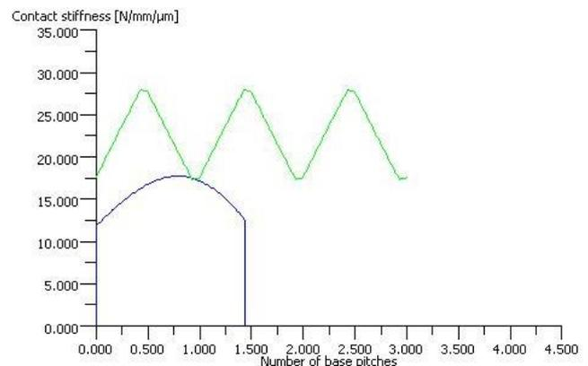
**Fig.1 - Initial contact stiffness for considered gear transmission**
