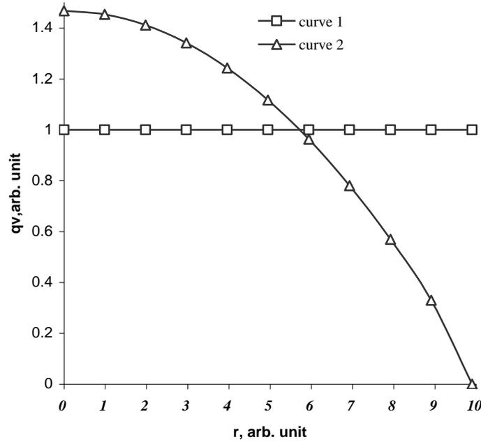
**Fig. 2.** Examples of qualitative radial distributions of volume power density in the cross-section of the laser tube of a pure copper vapor laser in relative units:  $\square$  - curve 1 ( $q_v(r) = q_0 = const$ ),  $\Delta$  - curve 2 of the type
