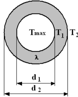
**Fig. 1.** Cross-section of the discharge tube of Cu laser:  $d_1 = 8.8mm$ ;  $d_2 = 10mm$ .
