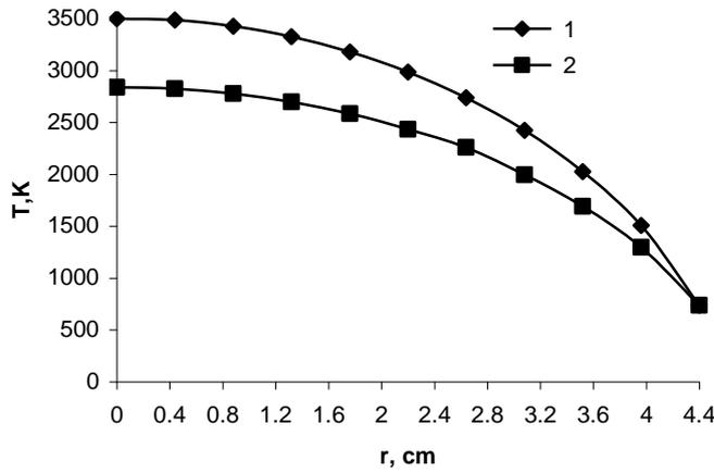
**Fig. 3.** Distribution of the temperature of the gas in the cross-section of a Cu laser: curve 1 – by formula (5); curve 2 – by formula (4).
