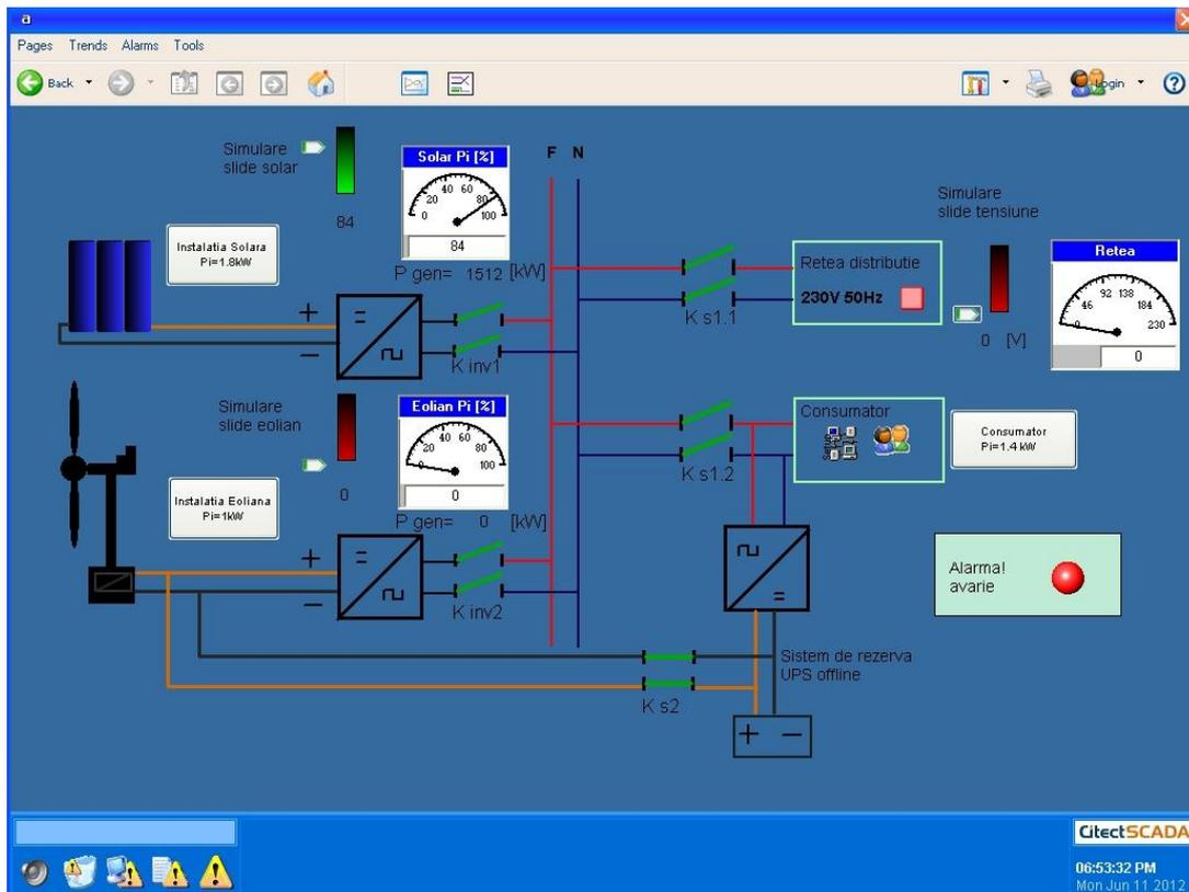
Fig. 5 – Alarm status of the hybrid solar-wind system implementation in SCADA
