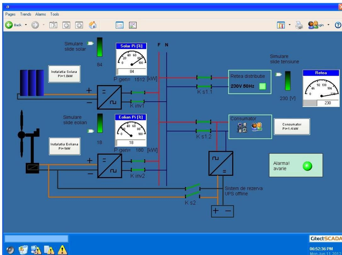
Fig. 4 – Permanent basis status of the hybrid solar-wind system implementation in SCADA
