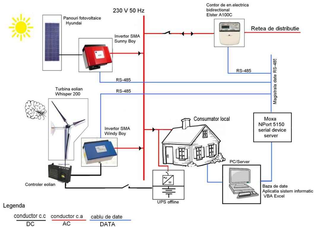
Fig. 3 – Hardware implementation of a solar-wind hybrid power system
