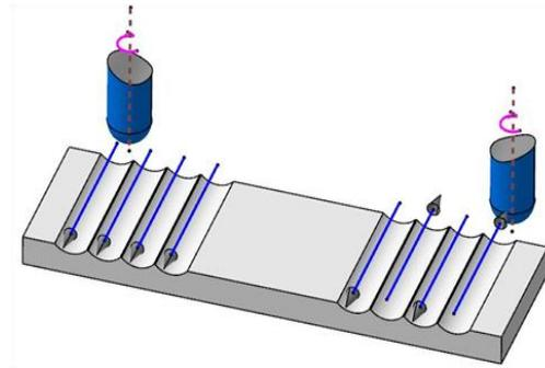
Fig. 3 Unidirectional and bidirectional finishing directions
