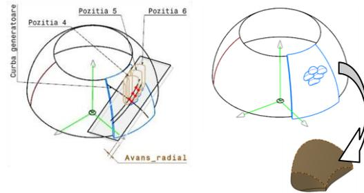
Fig. 6 Obtaining the geometry of the undetached chip
