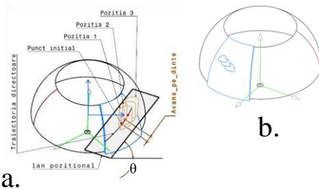
Fig. 5 Position of the cutting tool on the main feed path
