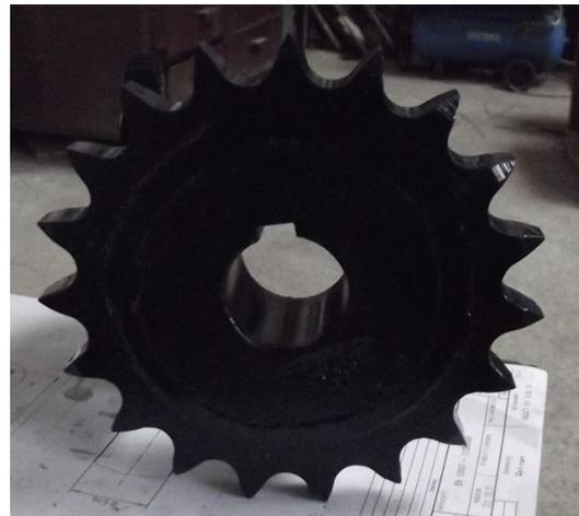
Fig. 9: Chain sprocket with 19 teeth [9], after the heat treatment of browning [14]
