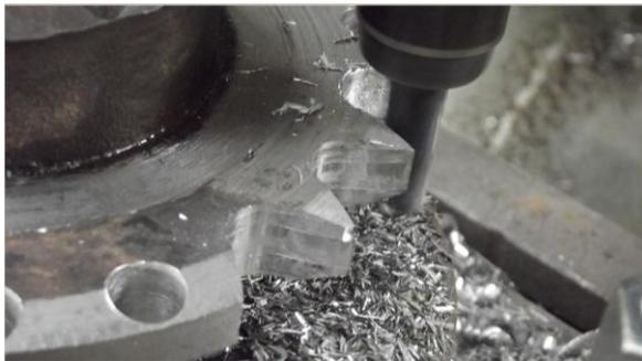
Fig. 7: It used the end mill  $\varnothing 12$  with 4 teeth at Roughing with subprogram P0155 [14]
