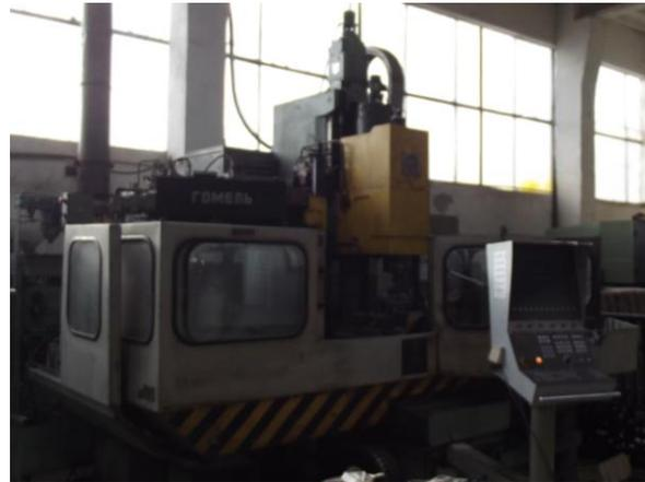
Fig. 1: GDV400PM1F4 vertical machining centers [14]
