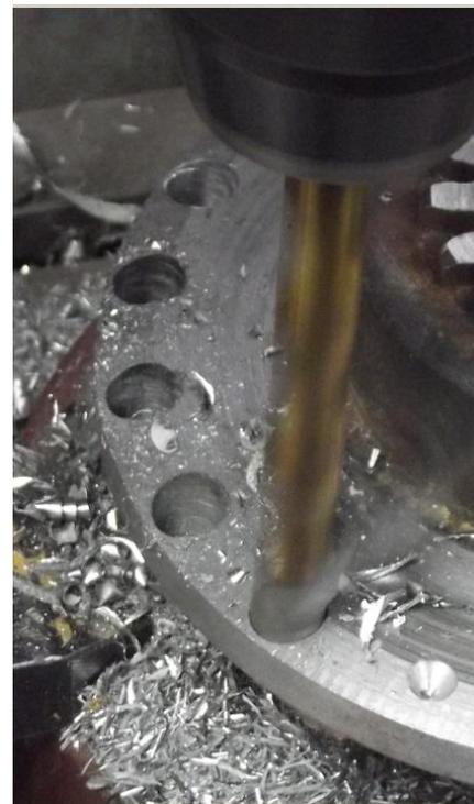
Fig. 6: Execution the holes of Ø12 with subprogram P0154 [14]
