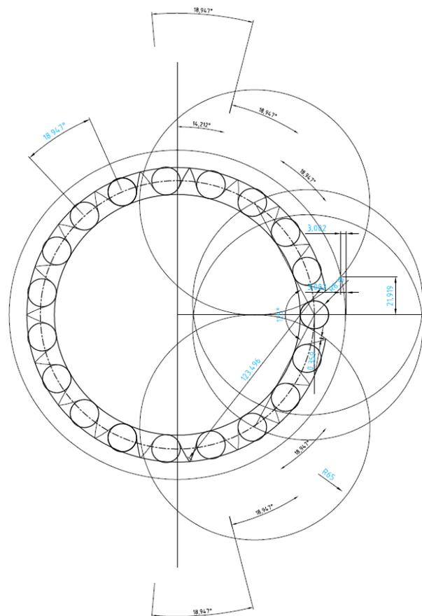
Fig. 3: Drawing sprocket with 19 teeth used to design processing program O0158 [10, 11, 12, 13]
