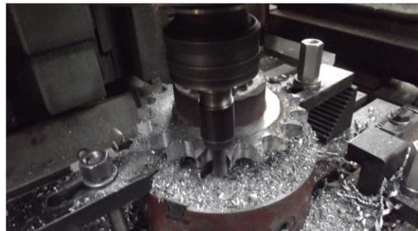
Fig. 8: Finishing toothing with end mill  $\varnothing 12$  having 4 teeth with subprogram P0156 [14]
