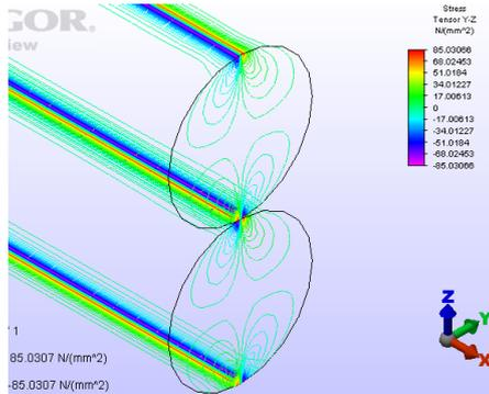
Fig. 15: Detail - Shear stress  $\tau$  distribution in the upper cylinder
