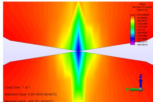
Fig. 8: Detail - Minimum principal stress  $\sigma_3$  distribution in contact area of the two cylinders
