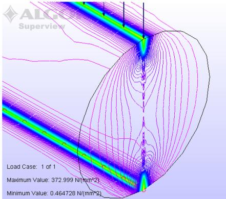
Fig. 10: Detail - Equal stress Von Mises  $\sigma_{ech}$  distribution in the upper cylinder
