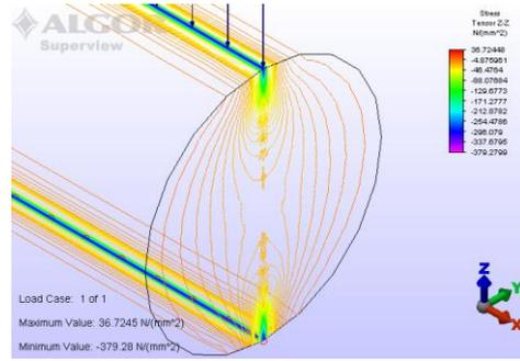
Fig. 13: Detail - Equal stress: Minimum principal  $\sigma_z$  distribution in the upper cylinder
