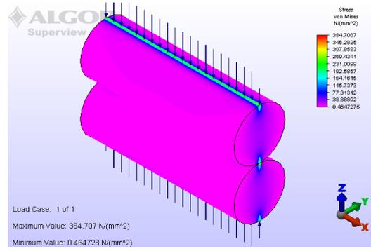
Fig. 5: Equivalent stress Von Mises  $\sigma_{ech}$  distribution in two cylinders
