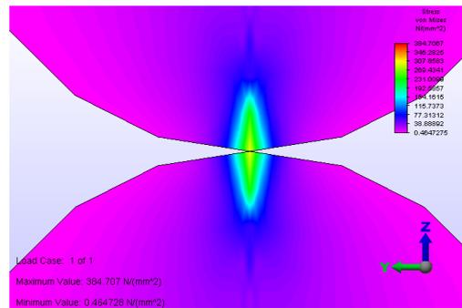
Fig. 7: Detail – Equivalent stress Von Mises  $\sigma_{ech}$  distribution in contact area of the two cylinders
