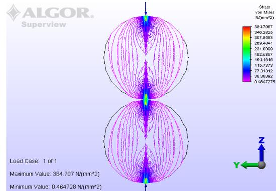
Fig. 6: Equal stress Von Mises  $\sigma_{ech}$  distribution in cross-section area of two cylinders
