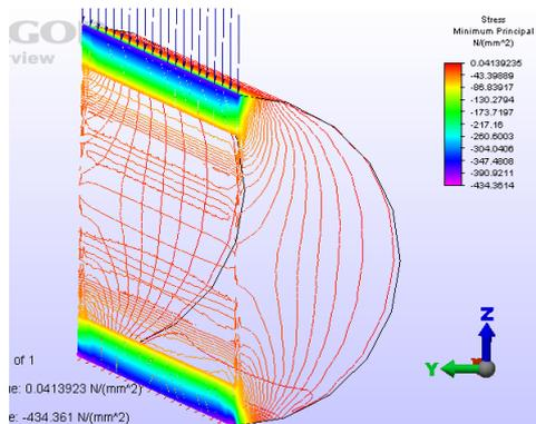
Fig. 12: Detail - Equal stress: Minimum principal stress  $\sigma_3$  distribution in the upper cylinder cross-section
