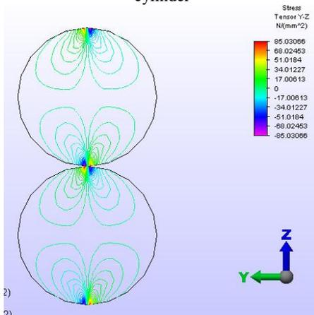
Fig. 16: Detail - Shear stress  $\tau$  distribution in the upper cylinder
