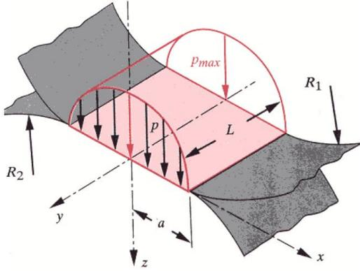
Fig. 3: Distribution of stresses in the contact area of two cylindrical bodies with parallel axes
