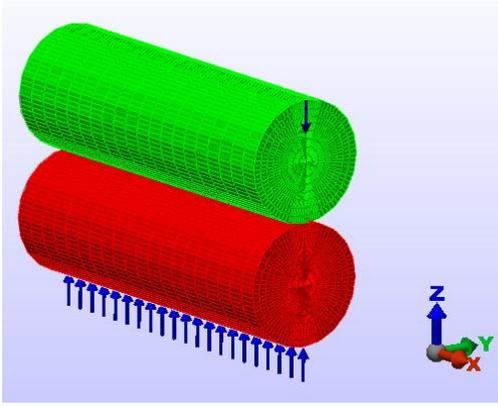
Fig. 4: Contact between two cylinders with parallel axes: Modeling and meshing
