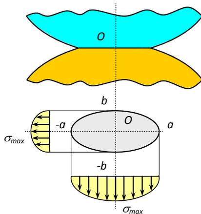
Fig.1: Contact between two bodies [2]
