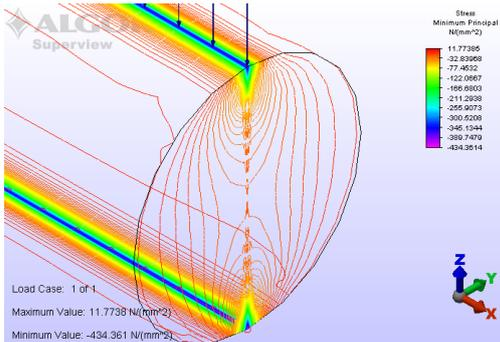
Fig. 11: Detail - Equal stress: Minimum principal  $\sigma_3$  distribution in the upper cylinder
