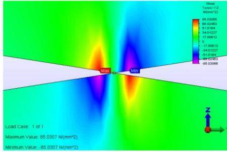
Fig. 17: Detail - Shear stress  $\tau$  distribution in the contact area of the two cylinders
