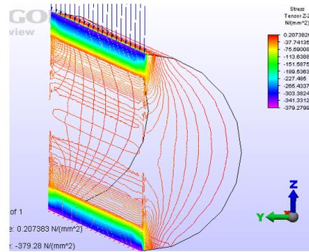
Fig. 14: Detail - Equal stress: Minimum principal  $\sigma_3$  distribution in the upper cylinder
