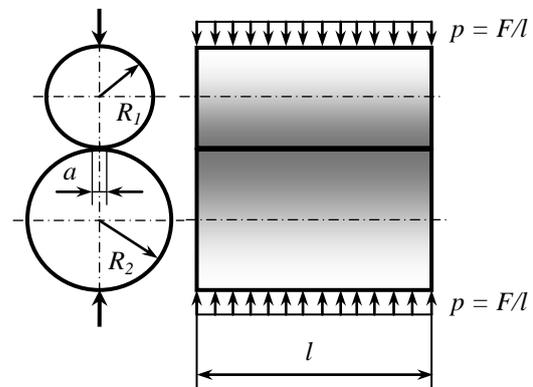
Fig.2: Contact between two cylinders with parallel axes
