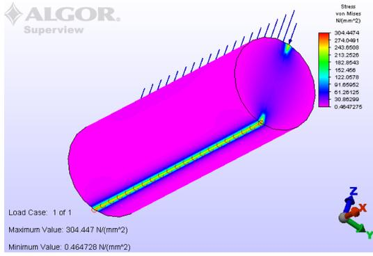
Fig. 9: Equivalent stress Von Mises  $\sigma_{ech}$  distribution in the upper cylinder
