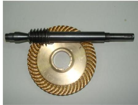
Fig. 6: Worm face gear with reverse tapered pinion
