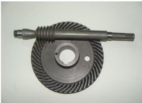
Fig. 4: Worm face gear with reverse tapered pinion
