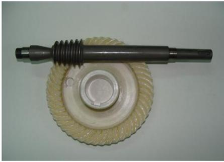
Fig. 2: Worm face gear with reverse tapered pinion
