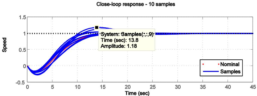
Fig. 8: The closed-loop response with:  $K_c = [1.136..1.388]$ ,  $T_{ws} = 2.75 \pm 20\%$  sec.,  $T_l = 10 \pm 20\%$  sec.
