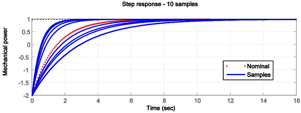
Fig. 3: The responses of an ideal turbine with  $T_{ws} = [0.5...6]$  sec. and  $T_{ws} = 2.75$  sec. as nominal value
