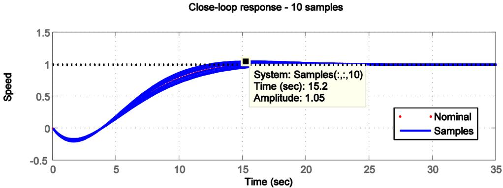
Fig. 7: The closed-loop response with:  $K_c = [1.136..1.388]$ ,  $T_{ws} = 2.75$  sec.,  $T_l = 10$  sec.
