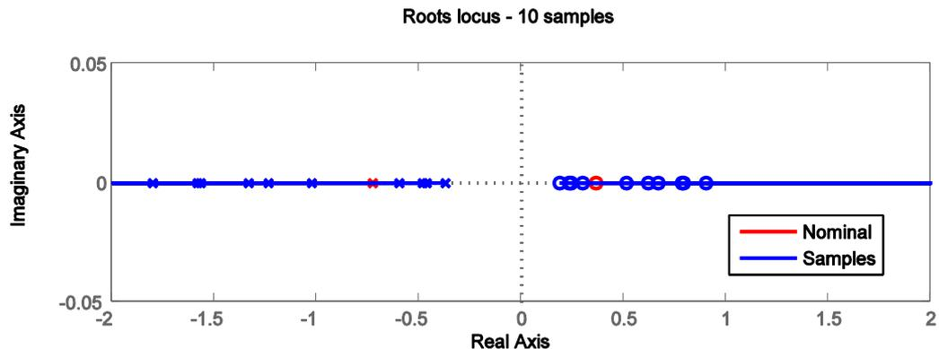
Fig. 2: Roots locus for of an ideal turbine with:  $T_{ws} = [0.5...6]$  sec. and  $T_{ws} = 2.75$  sec. as nominal value
