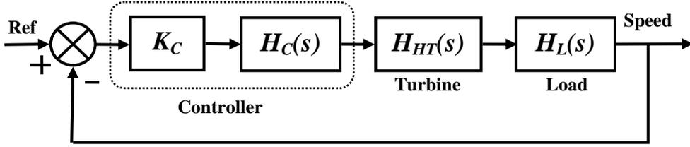
Fig. 6: The block diagram of the speed control
