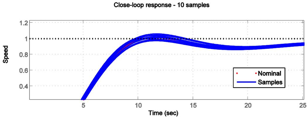
Fig. 9: The closed-loop response with:  $K_C = 1.250$ ,  $T_{WS} = 2.75 \pm 5\%$  sec.,  $T_I = 10 \pm 10\%$  sec.
