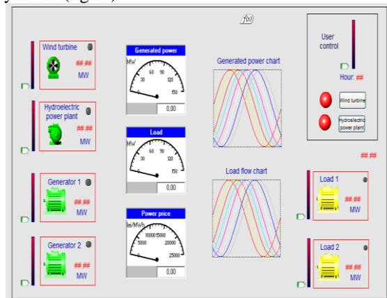
Fig. 5: Interface of SCADA system
