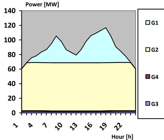
Fig. 6: Power dispatched by generators (DGs on-grid)
