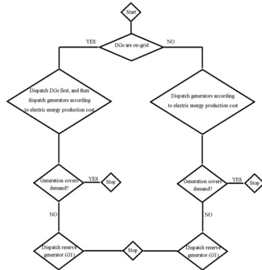
Fig. 4: SCADA simulation flow chart
