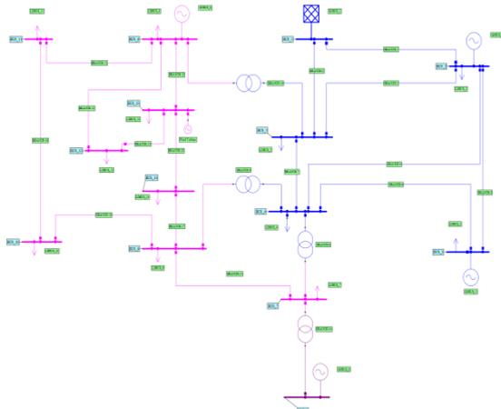
Fig. 3: One-line diagram of IEEE 14 system
