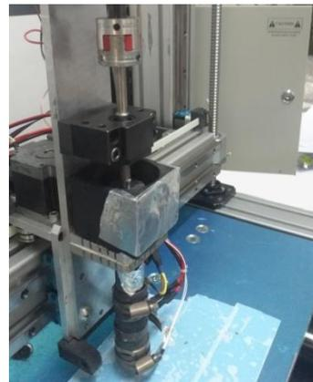
Fig. 9: Assembly extruder
