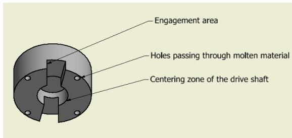
Fig. 6: The tapered piece
