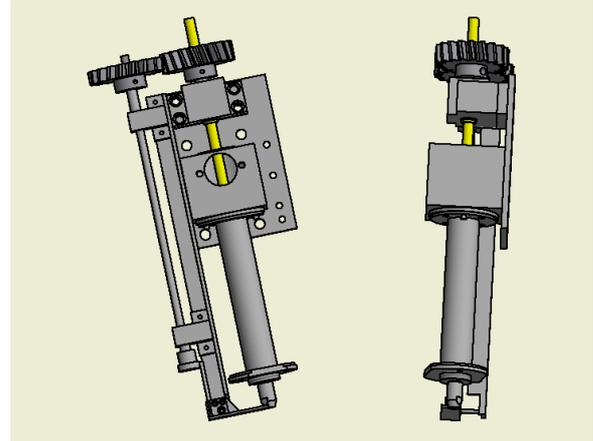
Fig. 3: Designed extruder
