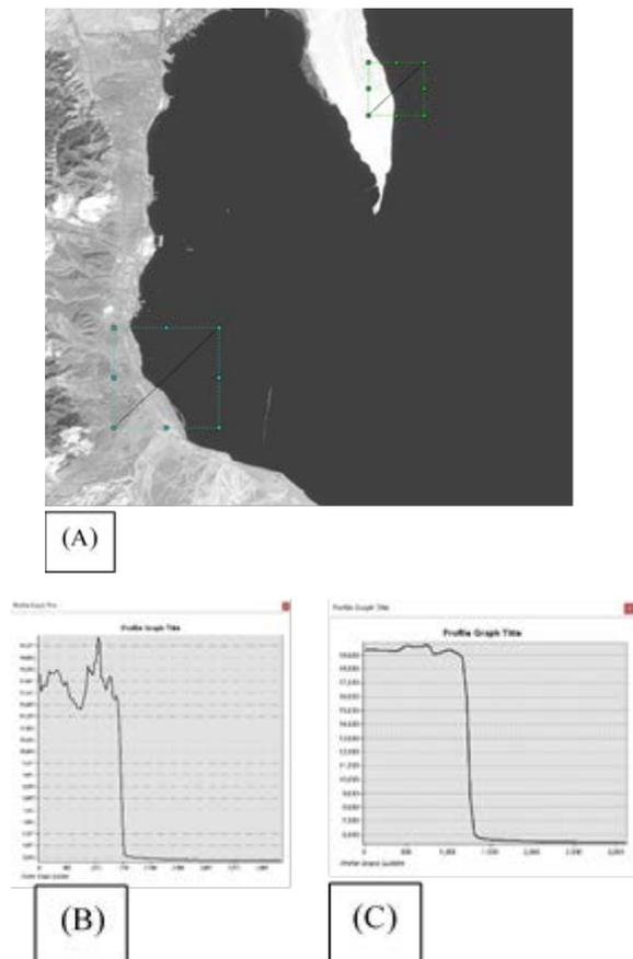
Fig 4: (A) INTERPOLATE lines created for Neari-nfrared band (B6); (B) and (C) Profile graphs for getting the average threshold value of SAFAGA satellite image for processing Water/ land separation.
