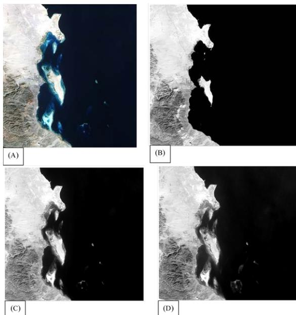
Fig 3: (A) MULTI true color of Landsat image of Safaga; and (B) Infrared Landsat image (band 6) of SAFAGA, Egypt; (C) Green band of Landsat image (band 3) of SAFAGA ; and (D) Blue Band of Landsat image (band 2) of SAFAGA.
