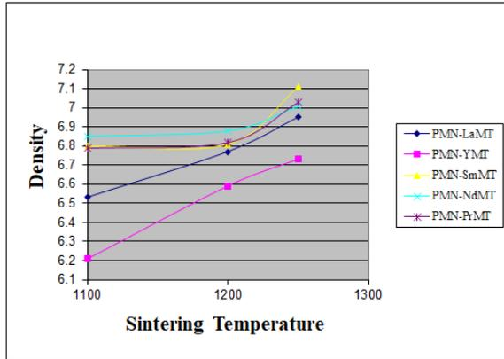
Fig.5: Variation of apparent density with sintering temperature of the  $0.9\text{Pb}(\text{Mg}_{1/3}\text{Nb}_{2/3})\text{O}_3 - 0.1\text{Ln}(\text{Mg}_{1/2}\text{Ti}_{1/2})\text{O}_3$  compositions
