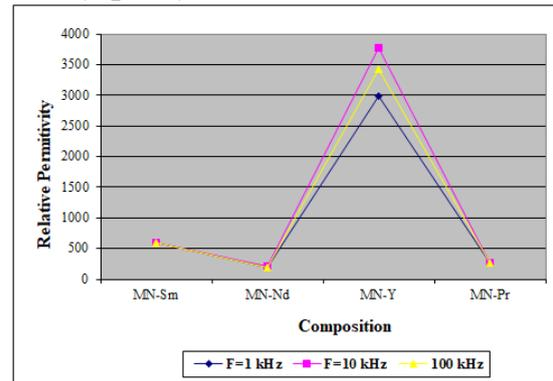
Fig.6: Variation of dielectric permittivity with composition at 1250°C
