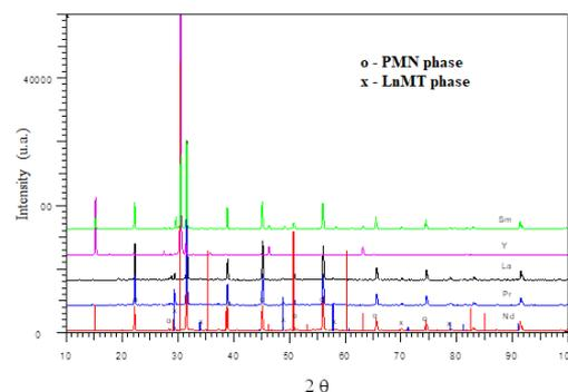
Fig.3: XRD patterns of  $0.9\text{Pb}(\text{Mg}_{1/3}\text{Nb}_{2/3})\text{O}_3 - 0.1\text{Ln}(\text{Mg}_{1/2}\text{Ti}_{1/2})\text{O}_3$  sintered 3h at  $1200^\circ\text{C}$
