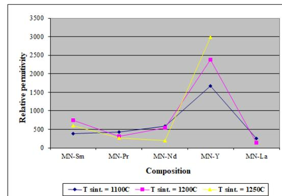
Fig.7: Variation of dielectric permittivity with composition at 1 kHz
