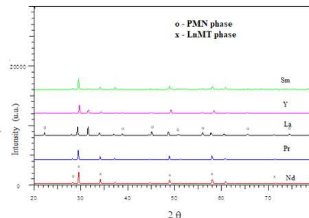
Fig.4: XRD patterns of  $0.9\text{Pb}(\text{Mg}_{1/3}\text{Nb}_{2/3})\text{O}_3 - 0.1\text{Ln}(\text{Mg}_{1/2}\text{Ti}_{1/2})\text{O}_3$  sintered 3h at  $1250^\circ\text{C}$
