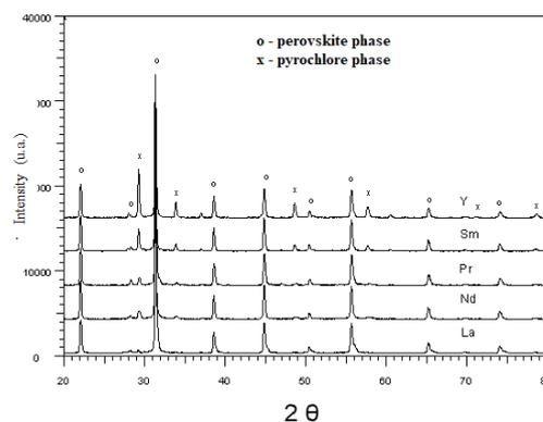
Fig.1: XRD patterns of  $0.9\text{Pb}(\text{Mg}_{1/3}\text{Nb}_{2/3})\text{O}_3 - 0.1\text{Ln}(\text{Mg}_{1/2}\text{Ti}_{1/2})\text{O}_3$  calcined 4h at  $870^\circ\text{C}$
