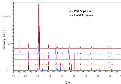
Fig.2: XRD patterns of  $0.9\text{Pb}(\text{Mg}_{1/3}\text{Nb}_{2/3})\text{O}_3 - 0.1\text{Ln}(\text{Mg}_{1/2}\text{Ti}_{1/2})\text{O}_3$  sintered 3h at  $1100^\circ\text{C}$
